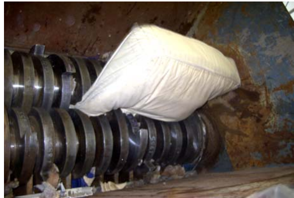
Conigliaro Industries, Inc. puts low-quality mattresses through a shredder (above), which separates the polyurethane foam from other materials. Below, brand name mattresses usually are filleted on each side and then run through the shredder, allowing the company to recycle a higher portion of material.
