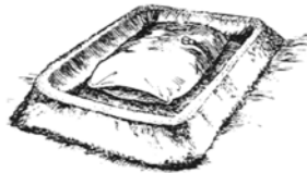
Figure 13. Freestanding Berm Protecting a Fuel Bladder.
