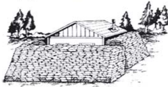
Figure 18. Sandbags against a Structure.
